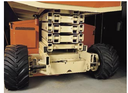
Strengthened Arm Stack for Improved Stack Rigidity
